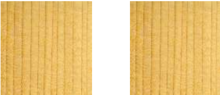
Fig. 12 Fiber orientation in relation to properly positioned cores (left), and improperly positioned cores (right) in core mounts
