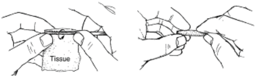
Fig. 10 Preparation to clean the borer (Jozsa, 1988).
