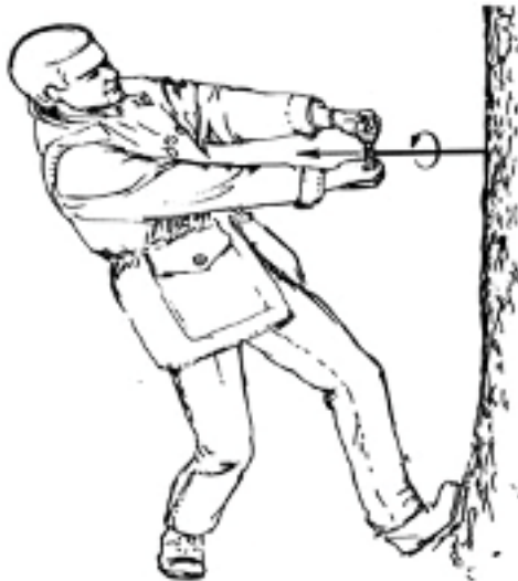
Fig. 7 Removing a struck borer (Jozsa, 1988).
