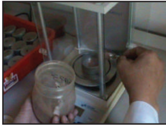
Fig.26 Weighing for moisture
