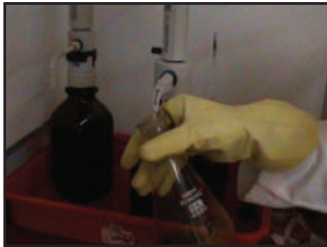
Fig.34. Adding sulphuric acid to sample
